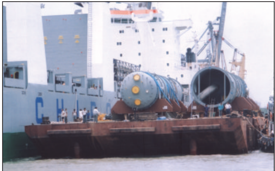
The reactors being carried by a barge (above) to the Chipolbrok vessel on to which it was deftly loaded (below)
